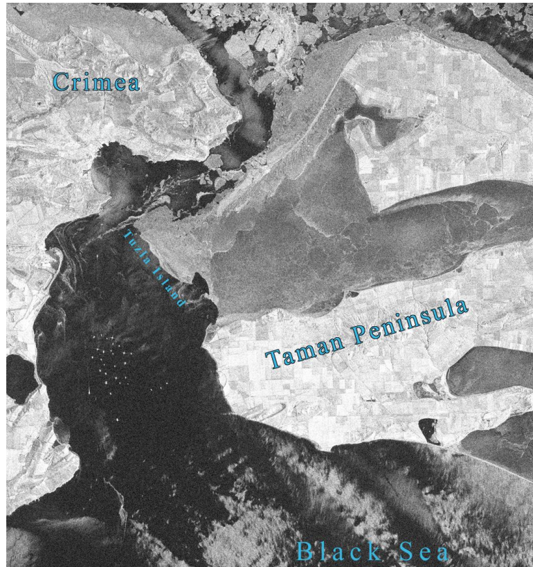
Figure 3. Ice cover in the Kerch Strait viewed by ERS-2 SAR, 21.01.2002 (VV polarization, pixel resolution 12.5 m).
