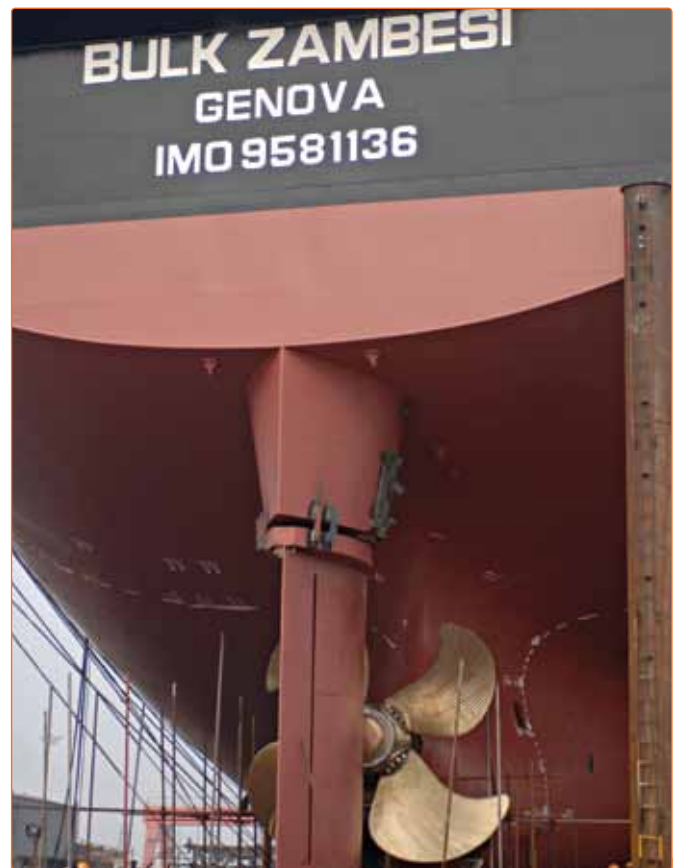
The rudder of the Bulk Zambesi is fitted with additional flap, making the vessel highly manoeuvrable.
