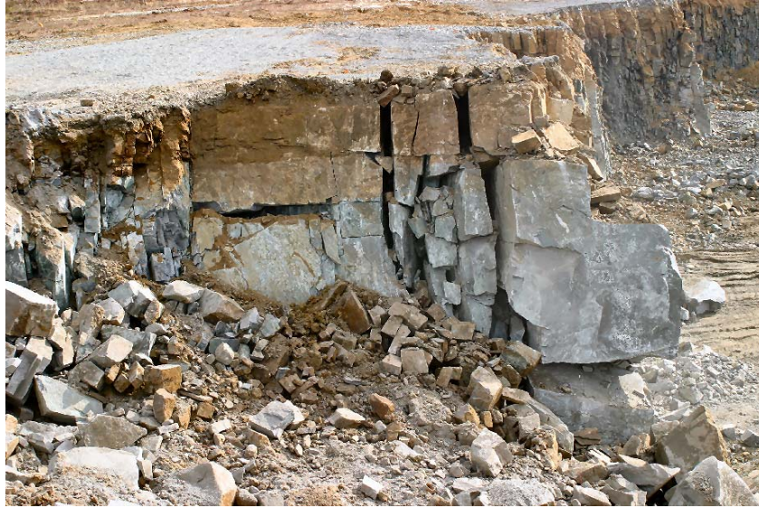
Figure 24. Liberated blocks in the back wall after the LS blast. These blocks are in the front face of the MTM blast.
