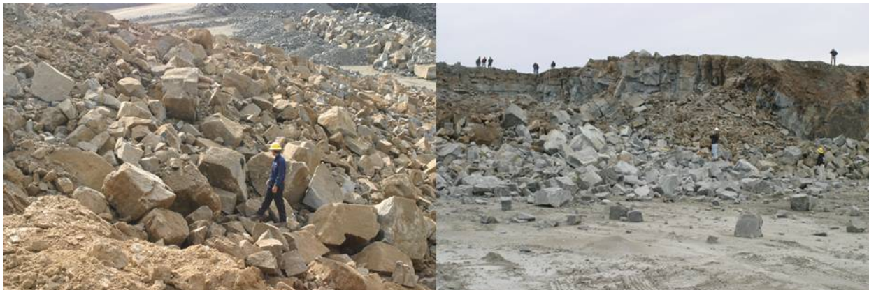
Figure 26. The surface of the LS (left) and MTM (right) muck piles – note the color of the oversize material.
