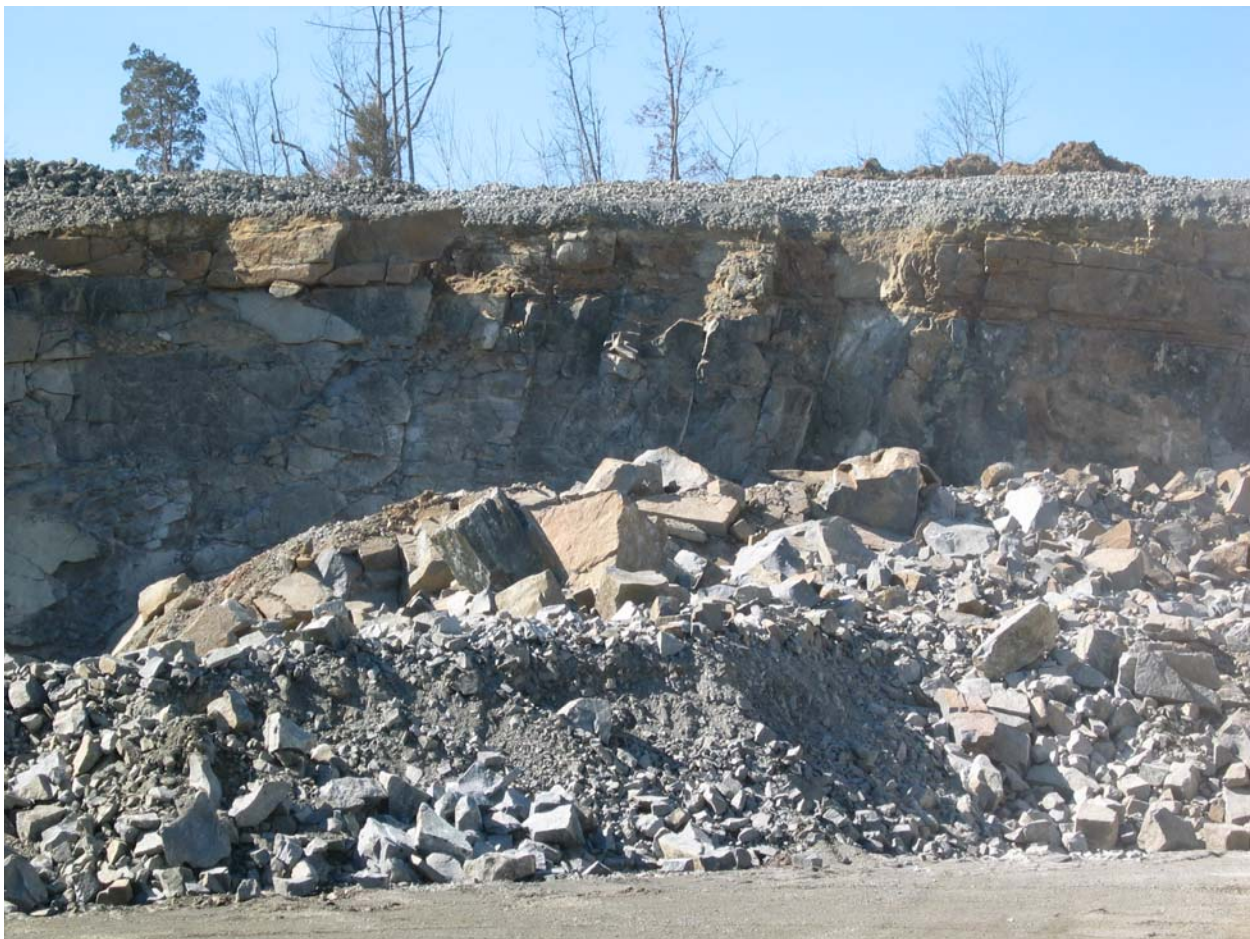
Figure 1. Photograph of the muck pile at the Bealeton Quarry showing large pieces of rock produced during blasting.
