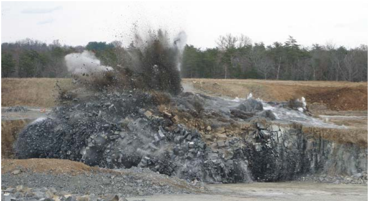
Figure 23. Photograph of the MTM blast clearly showing oversized blocks in the free face and stemming zones.
