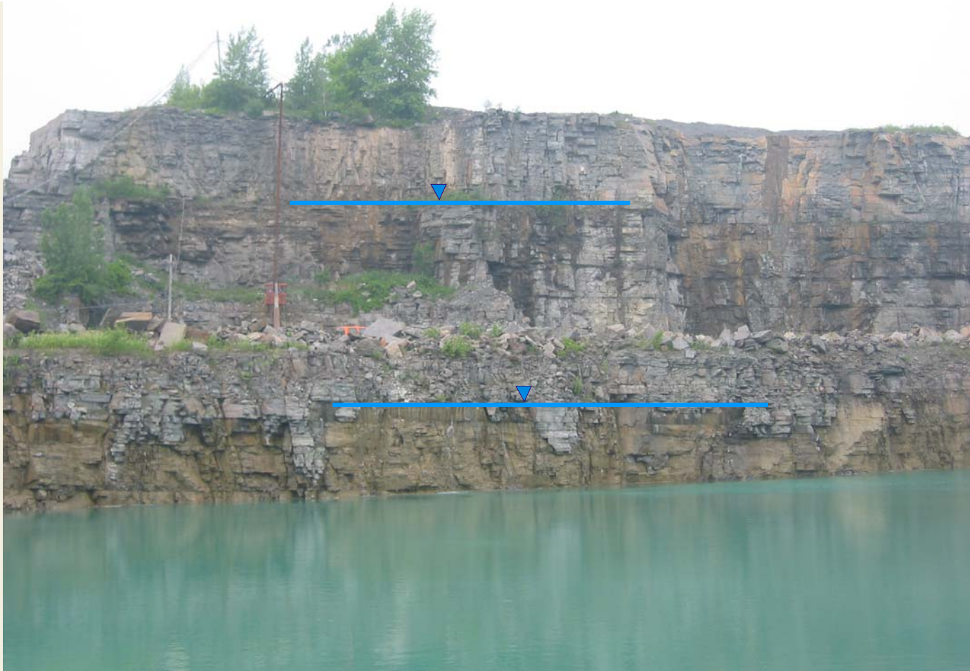
Figure 3. Seepage at Quarry walls
