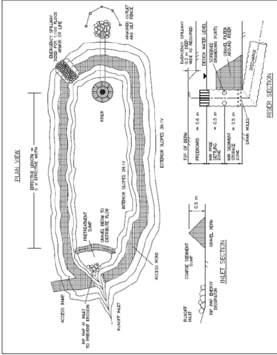
**Figure 2.5** Dry Detention Pond Plan and Sections as outlined in the Land Development Guidelines for the Protection of Aquatic Habitat, DFO (1993).
