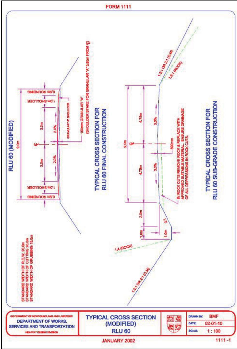
**Figure 2.3** Typical cross section of an RLU 60 road. Design as outlined in the NL Department of Works, Services, and Transportation Highway Design Specifications Book (2003).
