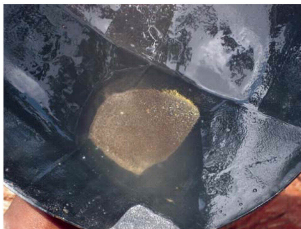
Figure 19. Gold is panned by the artisanal miners in an inner tube, near Kyereboso in Ghana in 2008. Field of view is approximately 30 cm.
