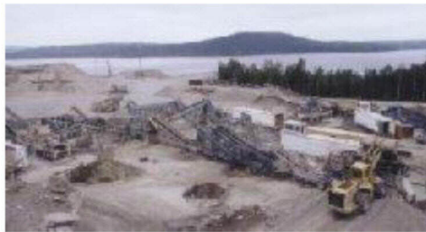
Layout of plant No. 2 with a Cat 988F feeding a Svedala 32x42 primary jaw crusher.
