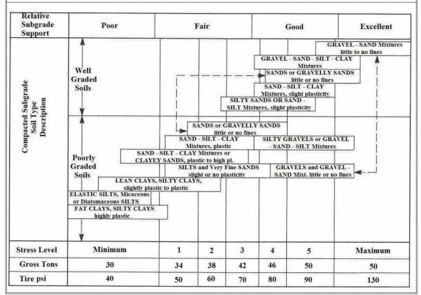
**D. Proof Rolling in Embankment Sections.** Immediately prior to final trimming of the subgrade surface and placement of subbase materials in embankment sections, all areas of the subgrade surface within roadway limits shall be proof rolled according to the requirements of this subsection. This work, and any delays due to this work, shall be considered incidental to the embankment item.
