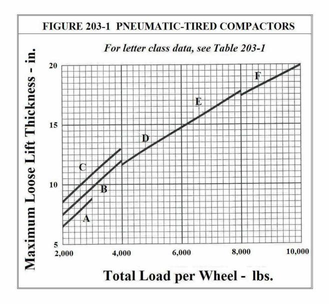
The minimum effort for all pneumatic compactors shall be 6 passes, at speeds up to 12 ft./sec on no more than the first 2 passes, and all subsequent passes at speeds of 6 ft./sec. or less.
