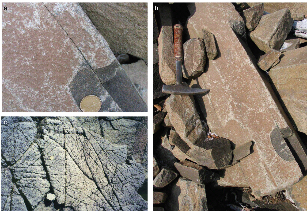
Figure 7a. Secondary sets of hairline fractures are commonly found in the columnar-jointed basalt. b. The large piece of columnar-jointed rock that is positioned diagonally across the photo contains two hairline fractures: one to the left of the hammer point and the other near the right edge of the piece of rock. c. Plan view of columnar-jointed basalt with pervasive secondary fracturing on Briar Island, Digby County. The fractures would project subvertically into the bedrock and sub-parallel to the long axis of the column block. This degree of fracturing would be unacceptable for dimension stone applications. One dollar coin for scale. d, e and f. (facing page). Examples of the tabular, blocky, prismatic and flagstone rock that were shaped by fracture systems.
