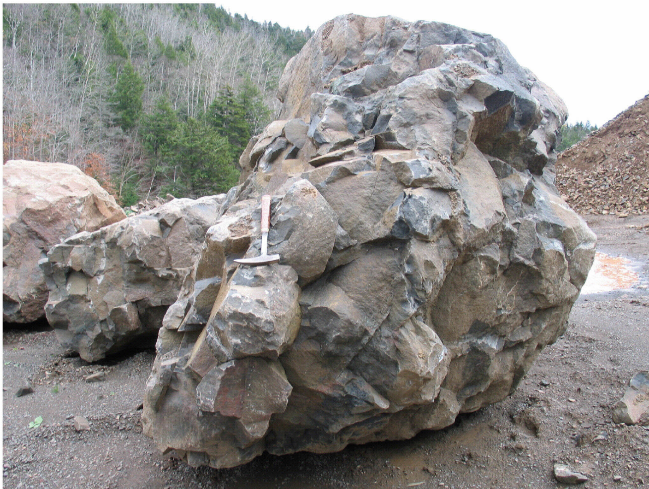
Figure 11. A large block of closely spaced columnar-jointed basalt that could be used for armourstone. It is unknown if this piece of rock would withstand the long term rigours of a marine tidal application. Would water eventually enter these sealed fractures, causing the rock to break down over time as a result of freeze-thaw cycles? Perhaps the placement of this type of rock in a structure such as a breakwater should be avoided because of the potential of premature failure.
