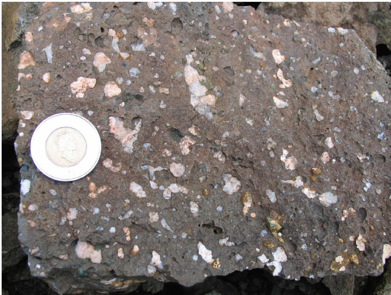
Figure 13a. Hand specimen of zeolitic basalt typical of the Middle Flow Unit.
