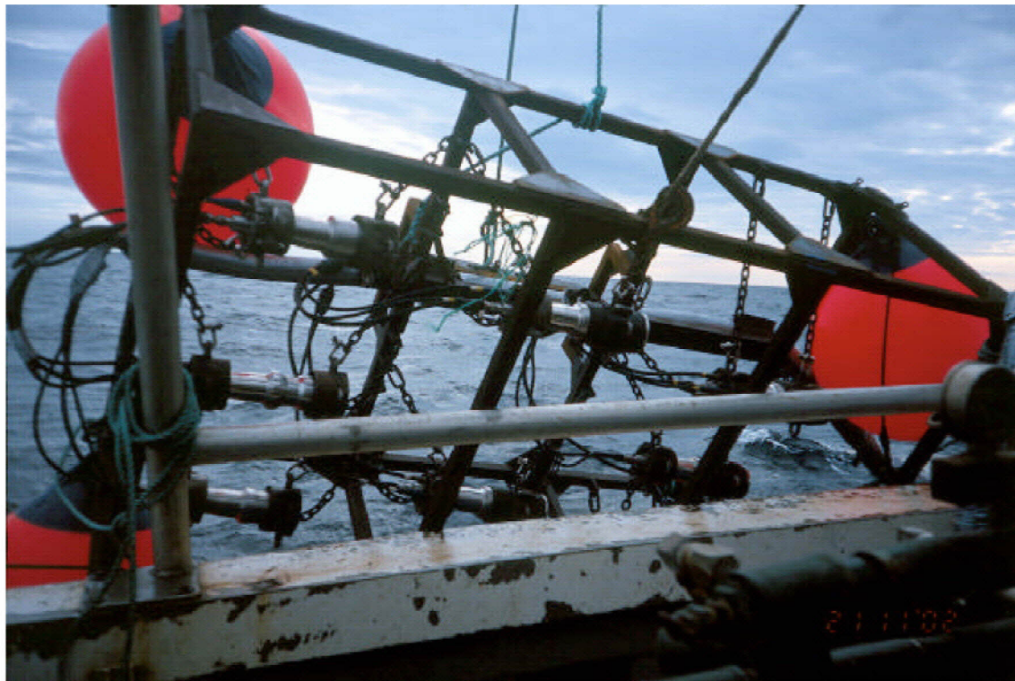
Figure 3. 200-in 3 seven-air gun array in frame.
