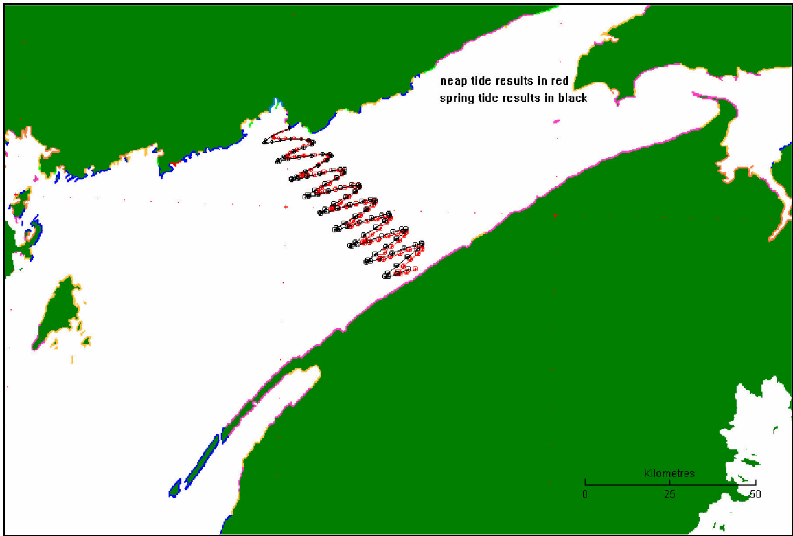
Figure 16.4 500 m 3 Diesel Spill at Marine Terminal: Winter Average Winds
