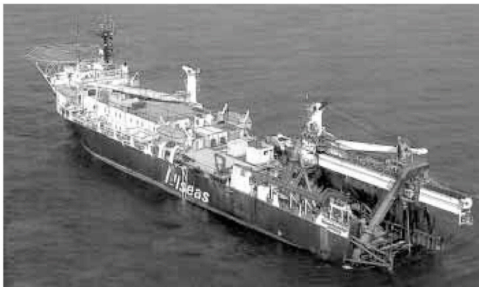
Figure 4. Photograph of a Typical Pipe-Lay Barge
