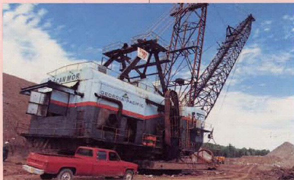
Top: Fiber gypsum board plant, Point Tupper. Above: 12 cubic yard dragline at Georgia-Pacific Corporation's Sugar Camp Quarry.
