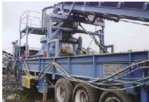
Svedala H6000 Hydrocone operating as the secondary crusher for plant No. 1.
