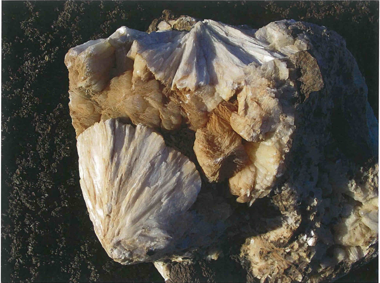
Figure 12. Specimen of stilbite, a common zeolite in the North Mountain Basalt and Nova Scotia's official mineral.
