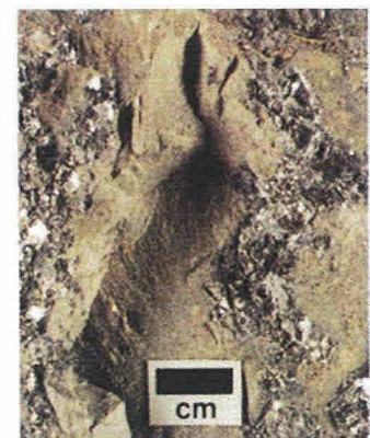
High-grade lead-zinc ore from the Gays River deposit.
