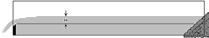
Figure 20-1 Portable Weir Box in Ditch
