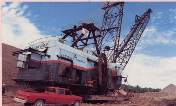
Top: Fiber gypsum board plant, Point Tupper. Above: 12 cubic yard dragline at Georgia-Pacific Corporation's Sugar Camp Quarry. Right: Loading fiber gypsum board at Halifax bound for Singapore.
