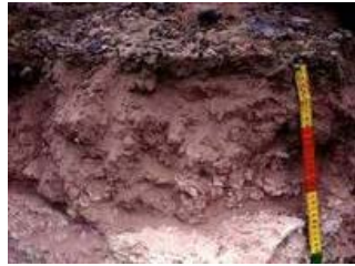
Calcisol with cemented calcium carbonate layer near to the surface in a desert environment, USA
