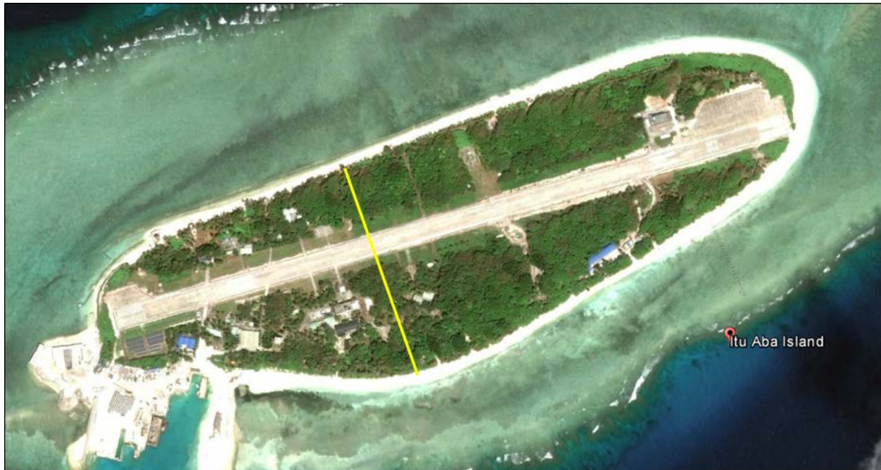
Figure 7. Cross-section (in yellow) for which the thickness of the freshwater lens was estimated for Itu Aba. The cross section is approximately 370 m
