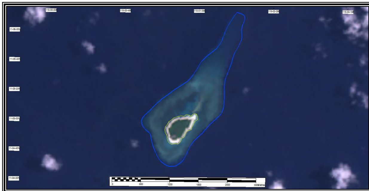
Figure 5.1.5: This is a 1:17,500 scale Landsat TM7 image with a 14.25 metre ground resolution dating from 21 April 2001. The image is in multi-spectral Band combination B3+B2+B1.
