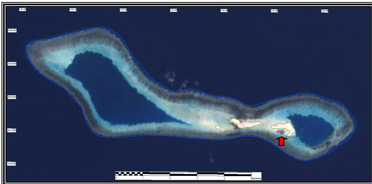
Figure 5.1.2: This is a 1:27,500 scale Landsat TM7, 14.25 metre ground resolution image, dated 26 November 1999 in multi-spectral Band combination of B3+B2+B1.
