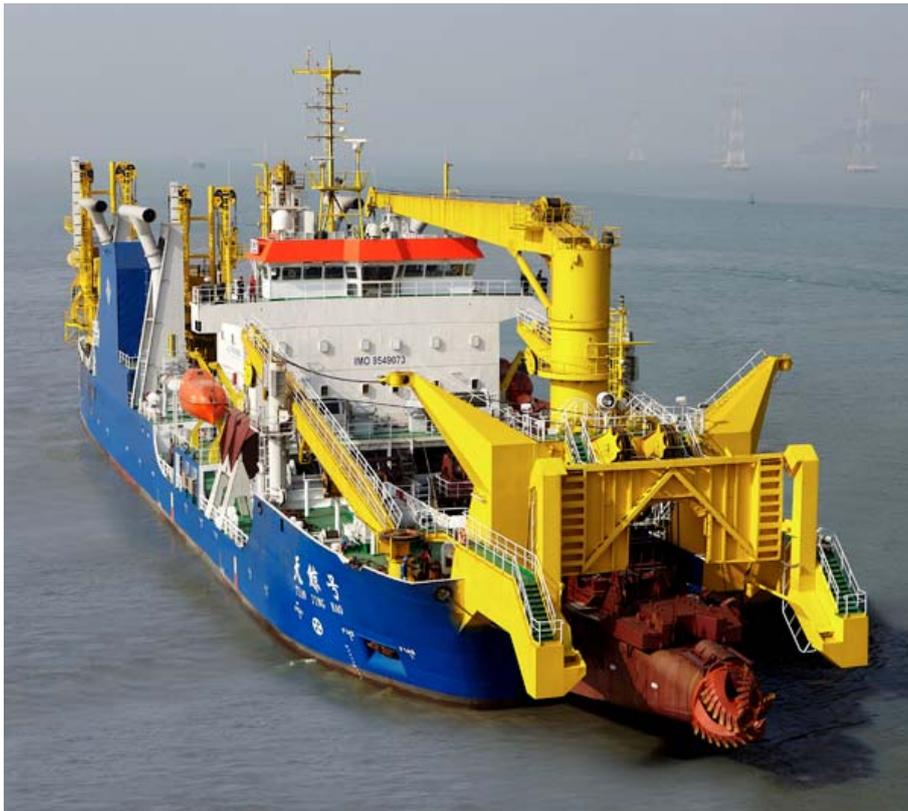
Fig 6: *Tian Jing Hao* is said to be the most powerful cutter suction dredger in Asia with a 4500 m<sup>3</sup> per hour extraction rate. Its length and width are 127.5m and 22m.
