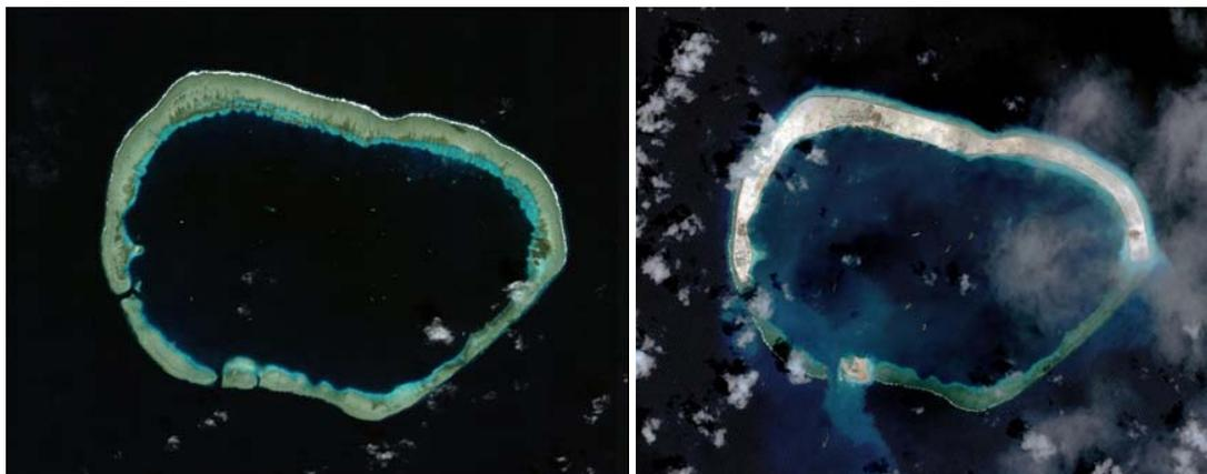
Fig 16: Mischief Reef. The picture on the left shows the atoll in its natural condition. The picture on the right, taken 8 September 2015 shows created land on top of nearly the entirety of the reef. The southern entrance of the atoll has widened to 275m. Picture source is DigitalGlobe, available via the CSIS Asia Maritime Transparency Initiative <http://amti.csis.org/mischief-reef/>.
