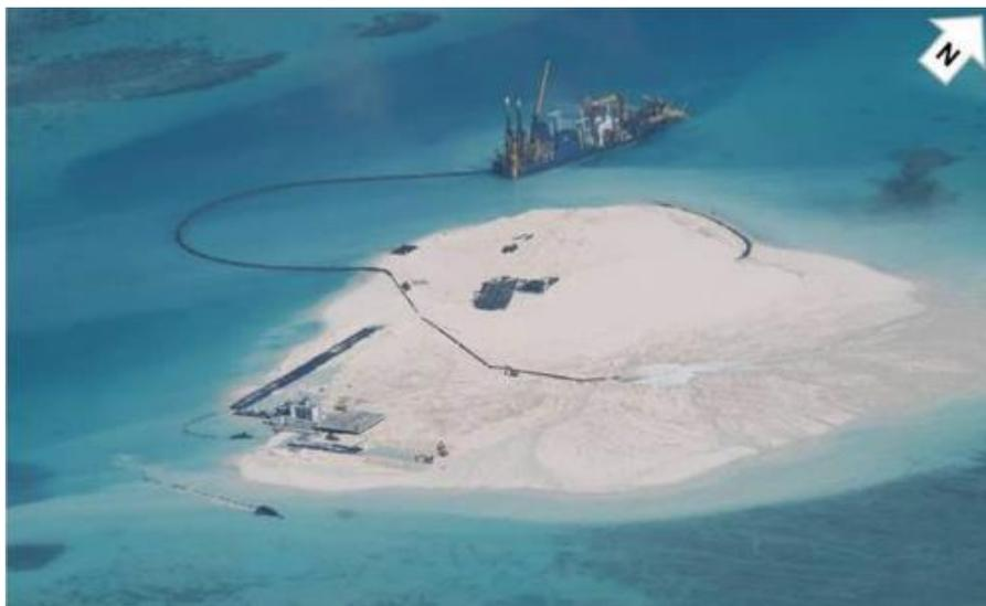
Fig 5: Land reclamation on Johnson South Reef on 25 Feb 2014. A dredger pumps spoils from the surrounding seabed onto the reef through a floating pipeline. Picture source: <http://www.dfa.gov.ph/index.php/2013-06-27-21-50-36/dfa-releases/2871-china-s-reclamation-on-mabini-reef>
