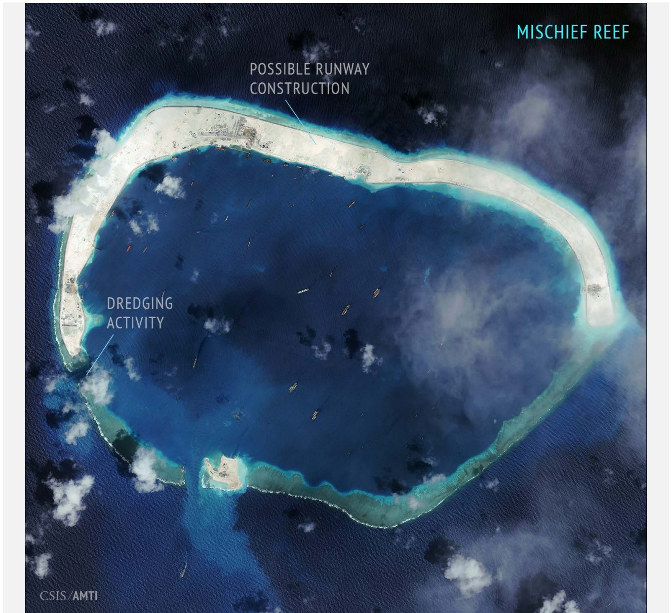
MISCHIEF REEF. September 8, 2015. A square area approximately 3,000 meters long has been cleared and flattened along the northern rim of the reef. Some believe an airstrip may be built in this straightaway in the near future. At the western access channel into the inner reef, an active dredger is visible. To the east, a second concrete plant has been set up on the rim of the reef.
