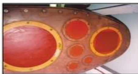
Figure 3. Mounting of EK 18, 38, 70, 120, 200 and 333 kHz echosounder on the drop keel of RV G.O. Sars
