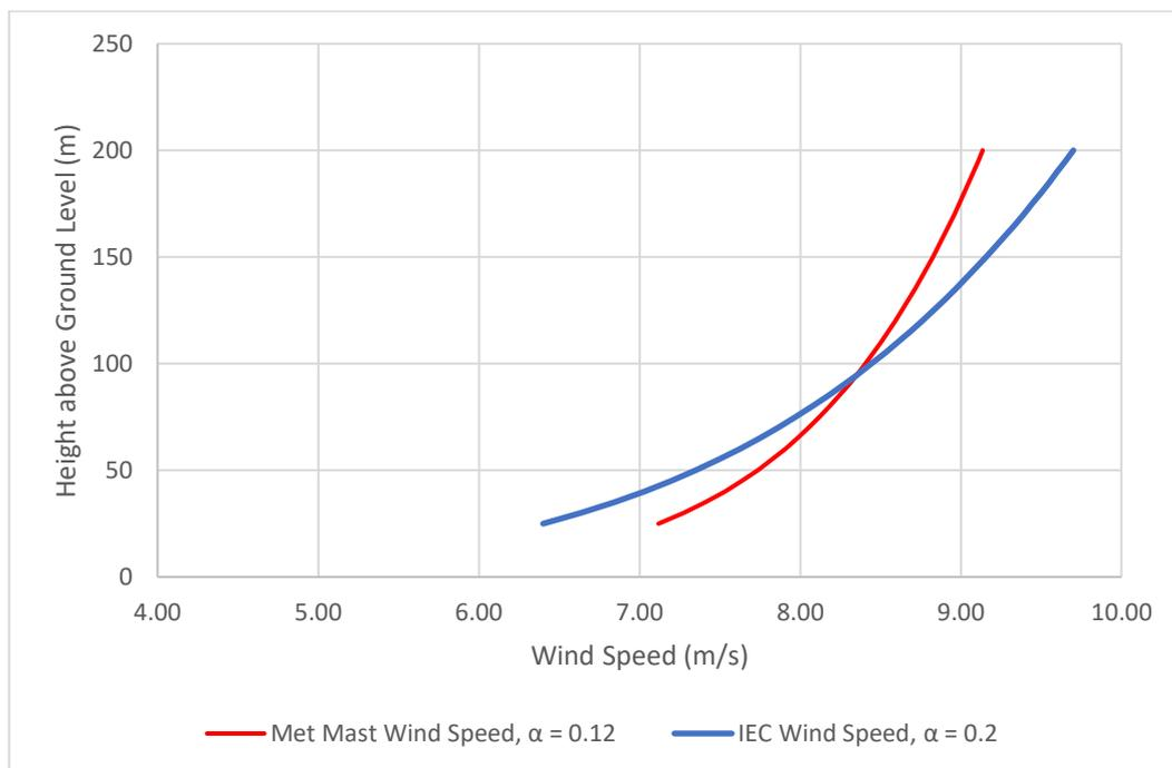
**Figure 3 – Site versus IEC Wind Shear Coefficient**
