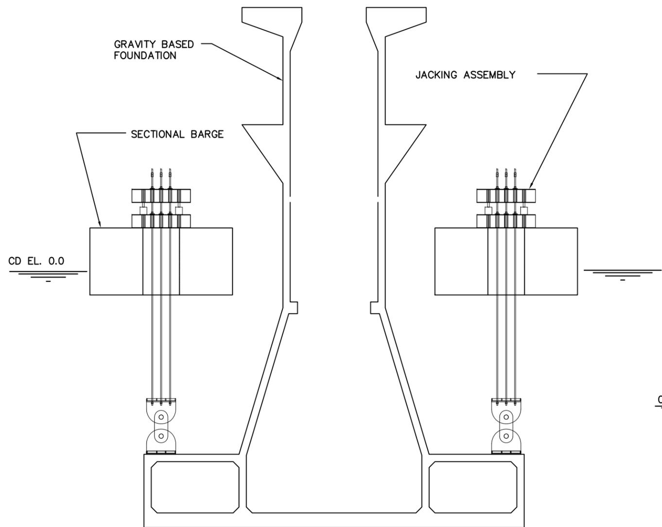
SECTION – BARGE & LIFT DEVICE
