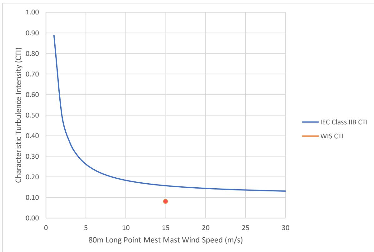
**Figure 2 – IEC Class II<sub>B</sub> CTI versus Wind Speed with Long Point Met Mast CTI at 15m/s**
