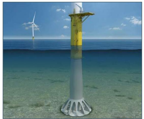
Figure 4-7 (Left): Borkum Riffgrund 1 suction foundation (Courtesy of Ørsted)
