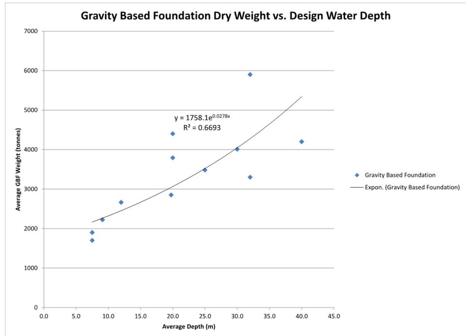
Figure 4-1: GBF Dry Weight vs. Design Water Depth
