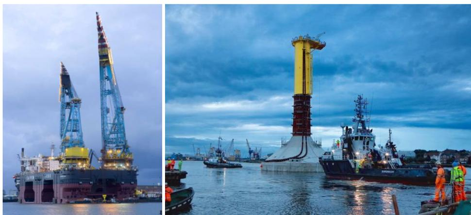
Figure 4. Saipem 7000 to be used for heavy lift installation at Fécamp (left) and float and sink installation by tug at Blyth (right)
