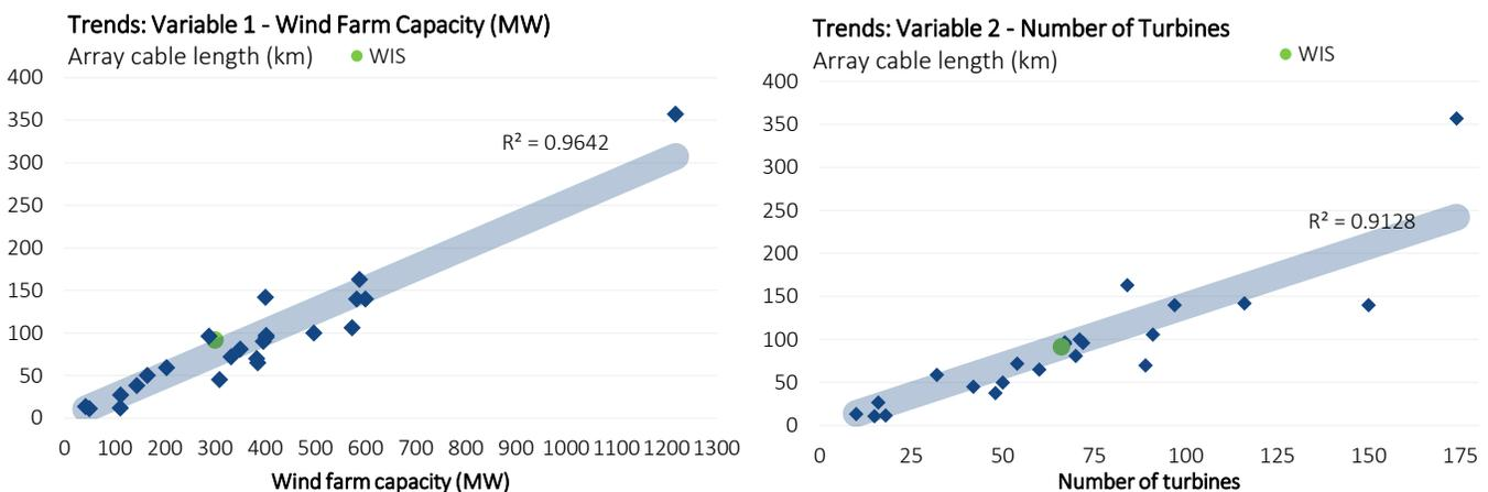
Figure 7. Multivariate array cable length model
