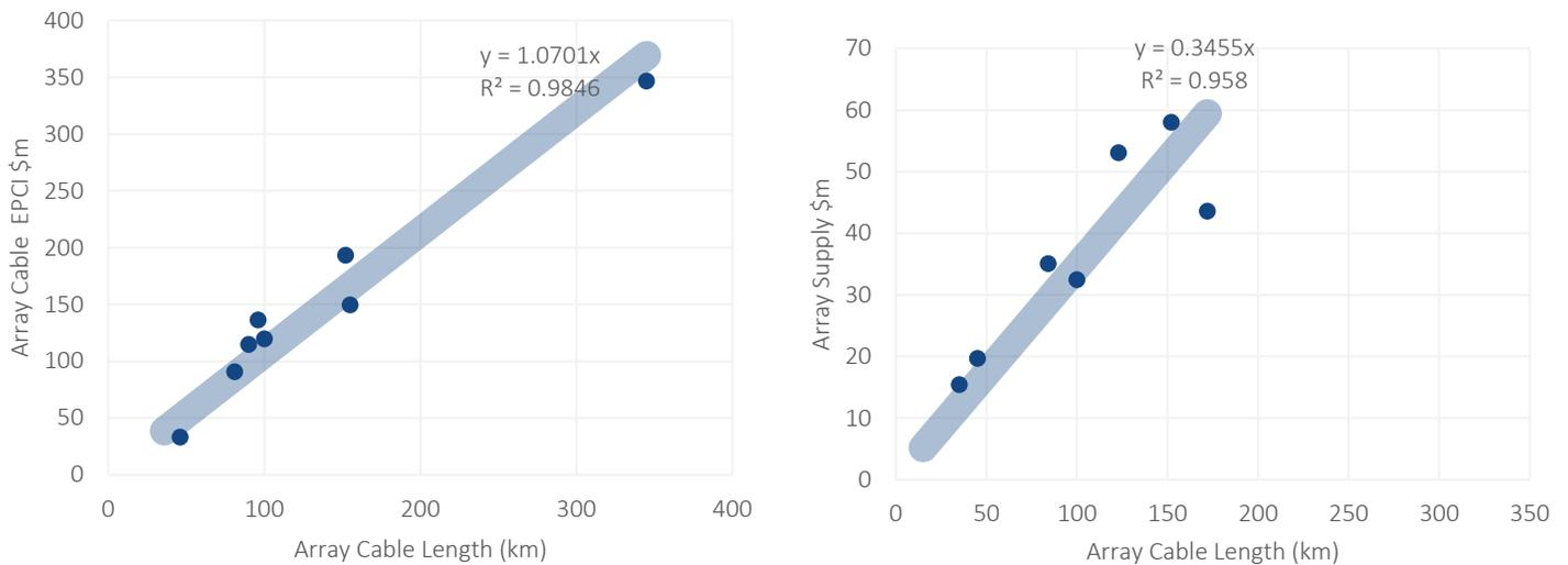
Figure 8. Cost model for array cabling
