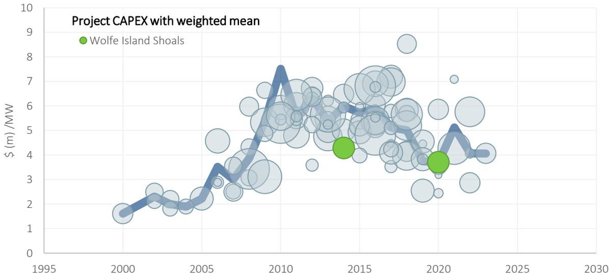
Figure 2. WIS project CAPEX in the context of European projects. Only showing projects >30 MW with bottom-fixed foundations that reached financial close prior to end-2020. Bubble size proportional to project capacity. In line with the dataset, WIS 2014 cost is not inflated to 2020.
