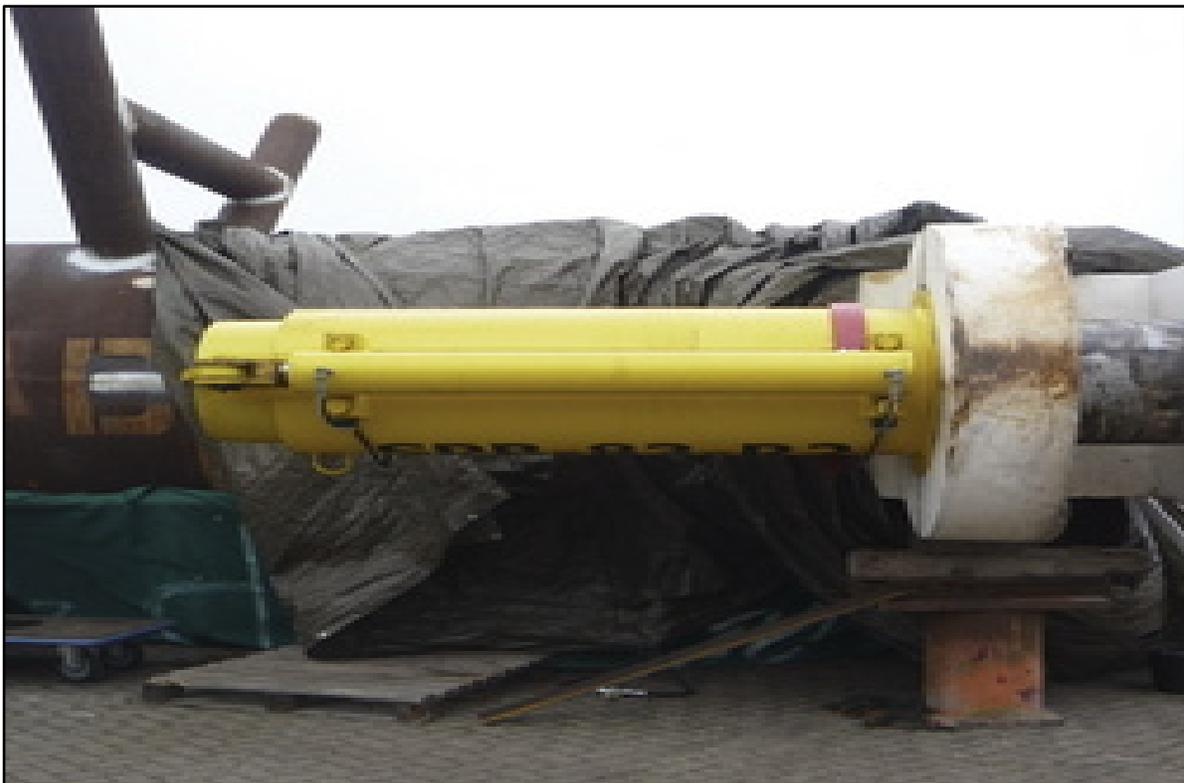
*Figure 1: Hydraulic Pin Release Mechanism*
