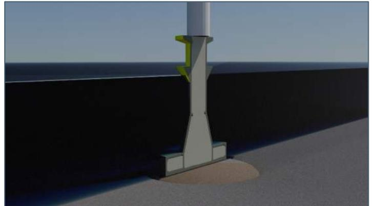
*Figure 5-2 (Right) COWI render of installed GBF section*
