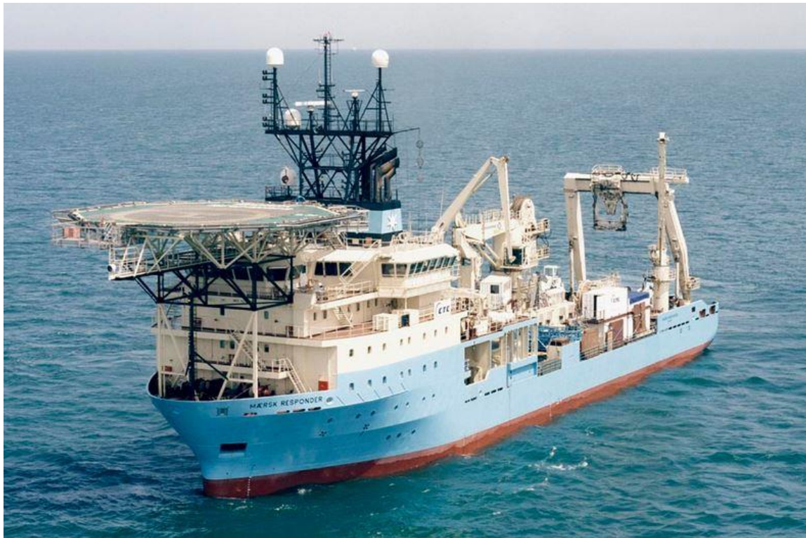
Figure 10-7: Cable Installation Vessel 12
