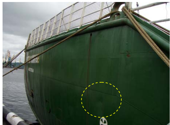
Slight dents on the shell plating
