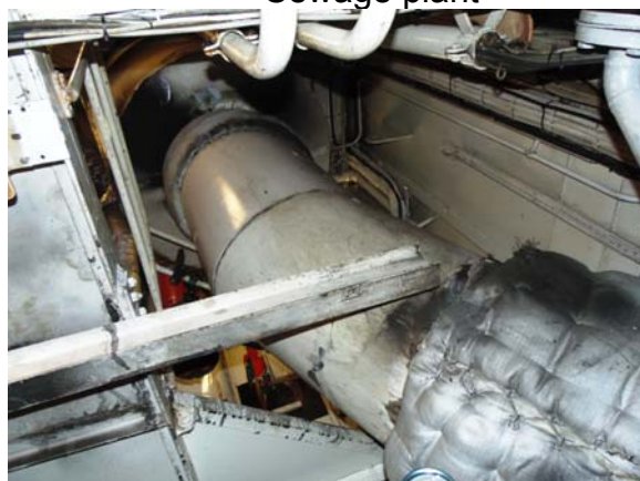
Main engine exhaust pipe
