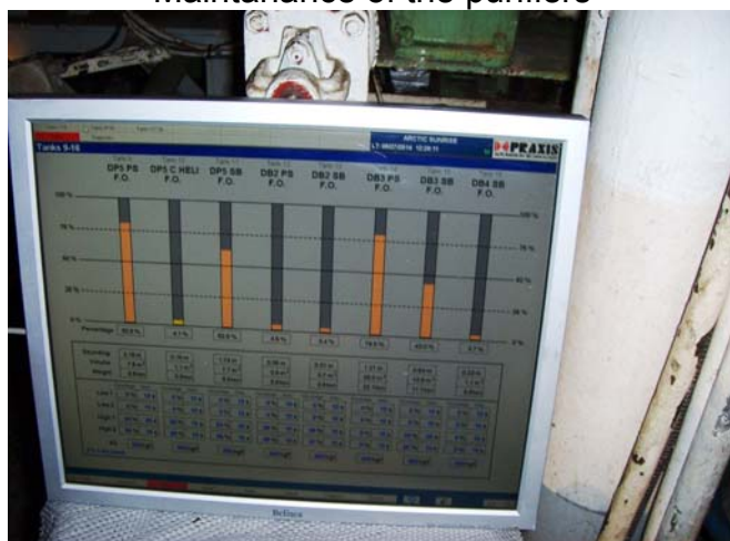
Monitor with the gasoil soundings
