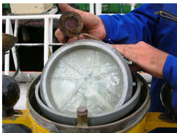
Magnetic compass is broken
