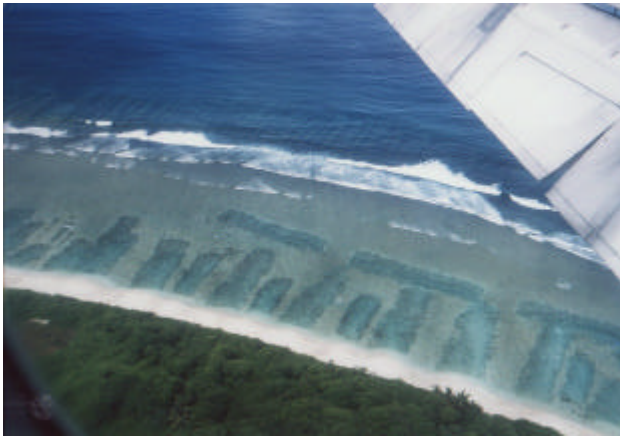
Figure 7.2 Sections of the seaward reef flat along the western side of the runway. Left: The rectangles are excavations of reef rock to about 1 m deep, made for the purpose of obtaining landfill. The reef crest is located where the waves are breaking. The much smaller perpendicular striations to seaward of the white water are the natural spur and groove system. Photo taken in 1966 by Prof. A. Eisenhauer. Right: Closer view of the northernmost extent, shortly after excavation. These perpendicular trenches extend right into the beach.
