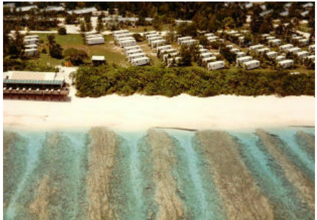
Figure 7.2 Sections of the seaward reef flat along the western side of the runway. Left: The rectangles are excavations of reef rock to about 1 m deep, made for the purpose of obtaining landfill. The reef crest is located where the waves are breaking. The much smaller perpendicular striations to seaward of the white water are the natural spur and groove system. Photo taken in 1966 by Prof. A. Eisenhauer. Right: Closer view of the northernmost extent, shortly after excavation. These perpendicular trenches extend right into the beach.
